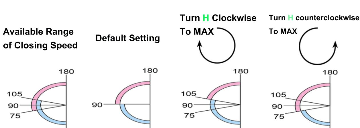
2. Adjustment of Closing Speed & Activate Any Degree Hold-Open in Closing Speed 2
