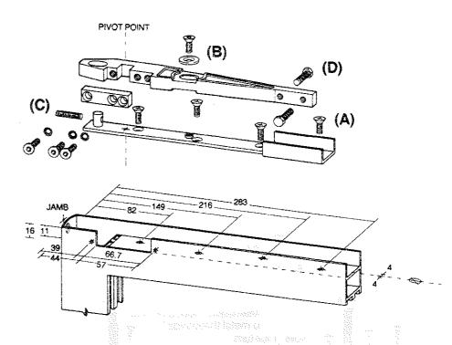
Prepare the top rail of the door as detailed, ensuring that the internal faces of the stile and top rail have been cut away to enable the closer spindle to be engaged during door hanging.
