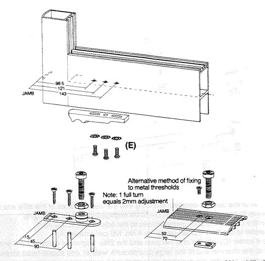
Prepare the bottom rail of the door to accomodate the pivot shoe with 2No. drilled and tapped M6 holes at 98.5mm and 143mm centres.
