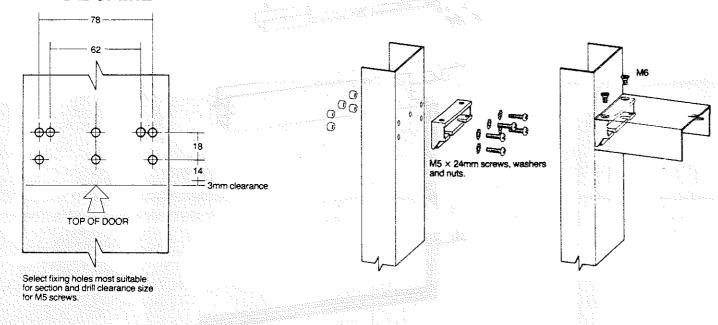
Prepare transom/header bar and cover plate to accept closer as detailed below. Fit jamb bracket to jamb with the 5 No. M5  $\times$  24mm screws, washers and nuts. Drill clearance holes and countersink header bar for 2No. M6  $\times$  10mm screws and 2No. M6  $\times$  15mm CSK bolts.
